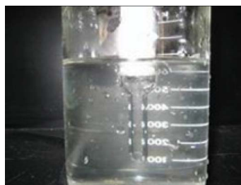
1—Column packed with the formulation is put in contact with a solution saturated in the water-soluble components of the formulation.
