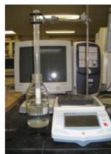
2—Scale and data collection system records the weight increase of the column as fluid permeates through the powder.
